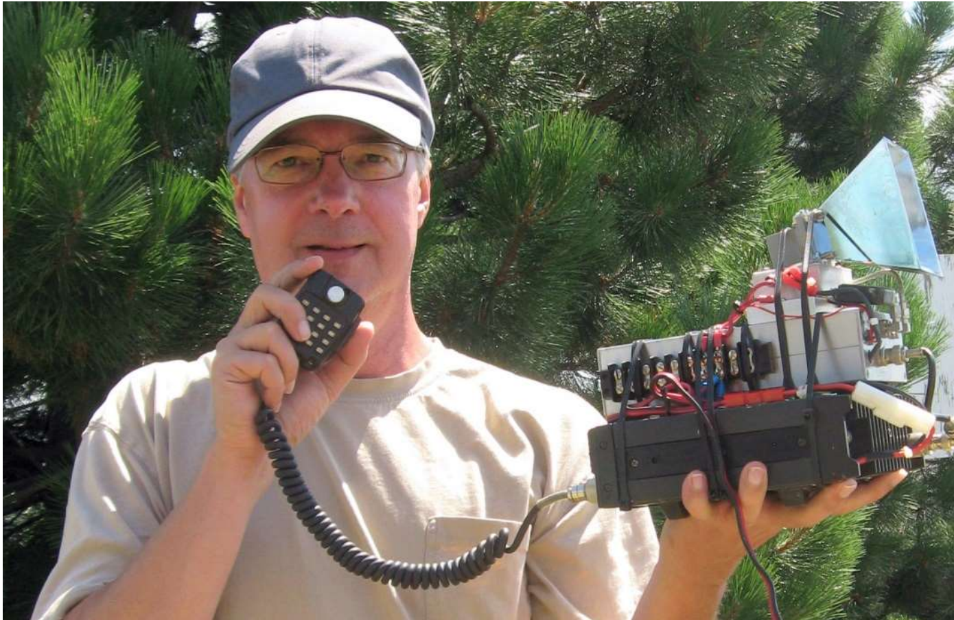
Jon Platt, W0ZQ, 10 GHz Horn Rig, 3 Watts Output, Buck Hill, 2014, ~150 mi QSO
